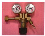
This certificate covers the homologation of the above-mentioned pressure regulators (see picture above). The classification, maximum inlet pressure, standard discharge and used gas are indicated above. The results of the homologation tests according to the above-mentioned standard are recorded in our reports L.32.332, L.32.416, L32.335, L.32.430, L.32.340 and L.42.775.
